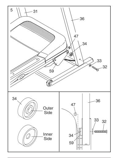
6. See the left inset drawing. Identify the outer side of the remaining Frame Spacer (34).
